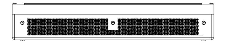
**Please note:**The grille size used in an IP3x anti-ligature radiator guard can inhibit the convection process. Therefore Contour cannot guarantee that the casing will not exceed a surface temperature of 43 degrees Centigrade.
